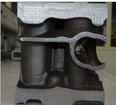
Figure 8. Cast Surface right after shot blasting
